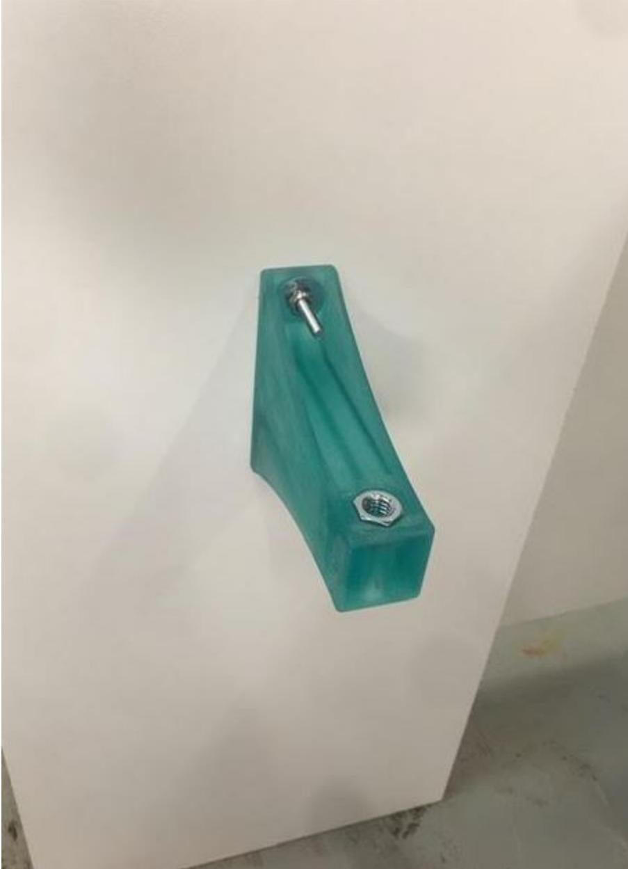
Install leg leveler by threading into 3/8" hex nut.
